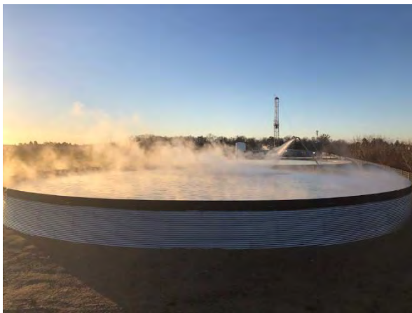
Figure 5: Thermal water trapped at the successful test in the well 'Essling-TH1', Vienna (photo: Austrian Geothermal Association, December 2021).
